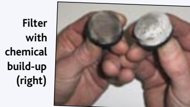
In-line strainer with deposit (left).
